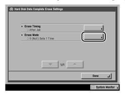
If the System Manager ID and System Password have been set, enter the System Manager ID and System Password using ⊚ - ⊚ (numeric keys) → press (Log In/Out).
