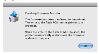
**11.** When the firmware is transferred, a message like the following is displayed on the printer Control Panel and the firmware is automatically overwritten. After the firmware has been overwritten, the printer restarts.
