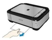
**6.** If any paper is sticking out of the Cassette, remove the paper, align and reload the paper in the Cassette.
