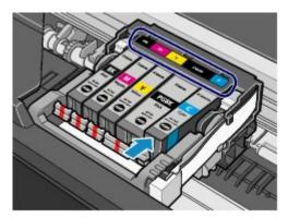
(2) Press the mark (Push) on the ink tank until the ink tank snaps firmly into place.
