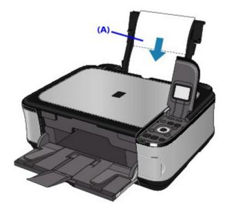
(A) Load the paper after unfolding it.
