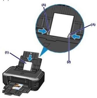
(1) Slide the Paper Guides (A) to open them, and load the paper in the center of the Rear Tray WITH THE PRINT SIDE FACING YOU.
