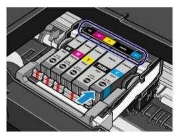
(2) Press the mark (Push) on the ink tank until the ink tank snaps firmly into place.
