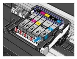
(2) Press the mark (Push) on the ink tank until the ink tank snaps firmly into
