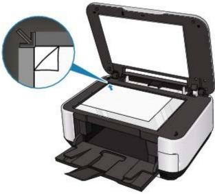
The Photo Index Sheet is scanned and the specified photos will be printed. Remove the Photo Index Sheet on the Platen Glass after printing is complete.
