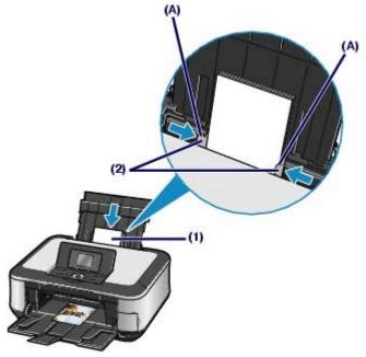
(1) Slide the Paper Guides (A) to open them, and load the paper in the center of the Rear Tray WITH THE PRINT SIDE FACING YOU.
