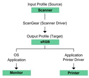
ScanGear (scanner driver) converts the image's color space from the scanner's color space to sRGB.
