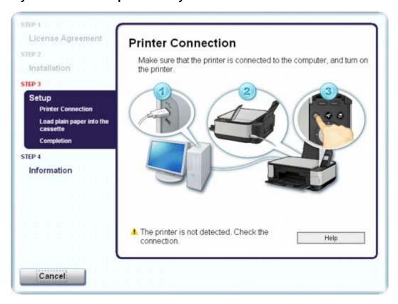
If you are unable to proceed beyond the Printer Connection screen, make sure that the USB cable is securely plugged into the USB port of the machine and is connected to the computer, and then
