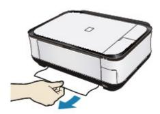
**6.** If any paper is sticking out of the Cassette, remove the paper, align and reload the paper in the Cassette.
