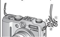
Pull the strap tight in the buckle so that it does not slip. Perform the same steps on the other side of the camera.
