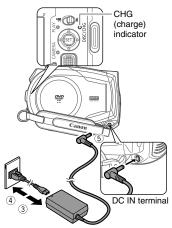
**3** Connect the power cord to the compact power adapter.
