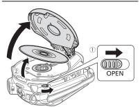
1 Slide OPEN fully in the direction of the arrow and gently open the disc cover completely until it stops.
