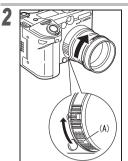
Attach the conversion lens adapter to the camera by aligning the part of the adapter marked (A) with the ring release button, then rotating it until the  $\bigcirc$  mark.
