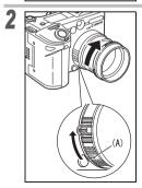
Attach the adapter to the camera by aligning the part of the adapter marked (A) with the ring release button, then rotating the lens adapter until the part marked (A) aligns with the  $\bigcirc$  mark.
