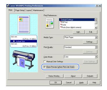
During printing, the PageComposer is displayed. Select the name of the document to be printed, and check the image displayed in Preview.
